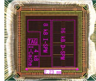
Fig. 1. Chip photograph of the fabricated RISC processor in a 65-nm FD-SOI process technology.
