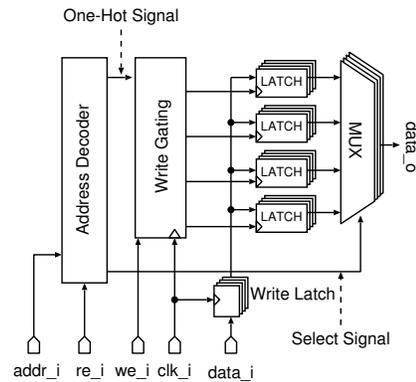
Fig. 2. Standard-Cell based Memory (SCM) structure.
