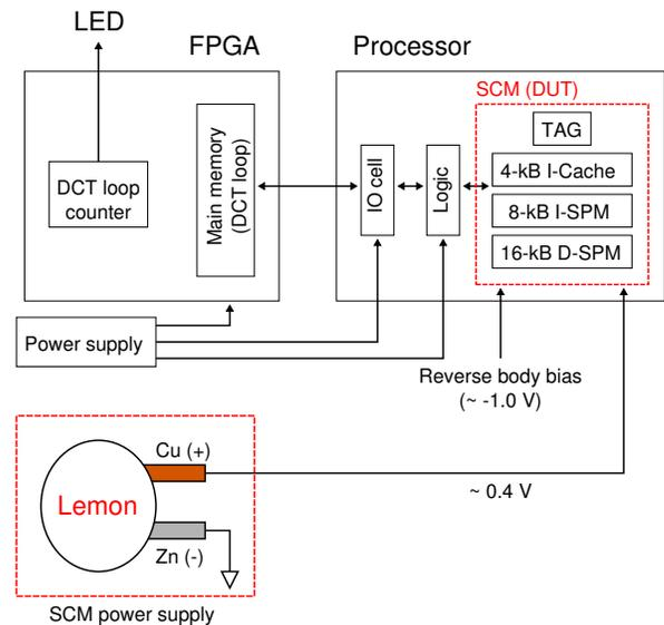
Fig. 3. Demonstration circuit.
