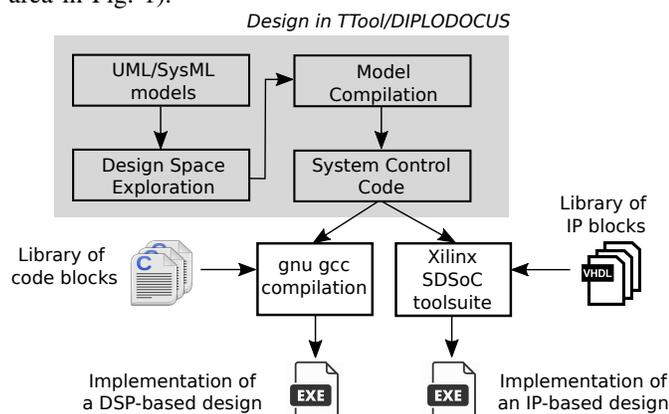
Fig. 1. Our approach for the design of 5G mixed-architecture solutions
