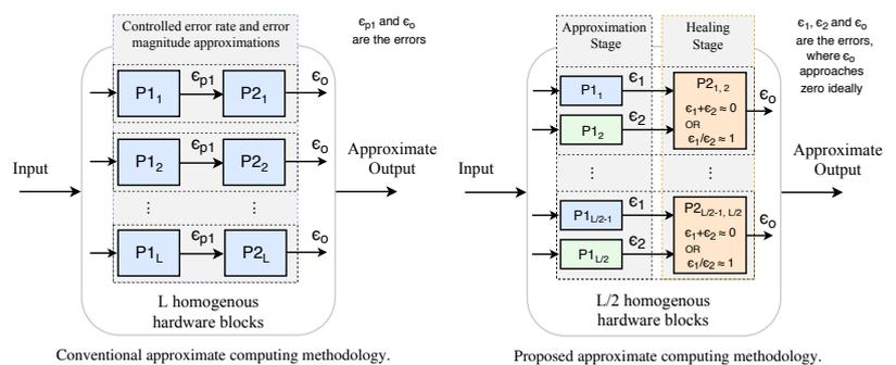
Figure 3. The proposed self-healing methodology [5] does not restrict the approximations based on an error profile but provides the opportunity for error cancellation to achieve an effective quality-efficiency trade-off.
