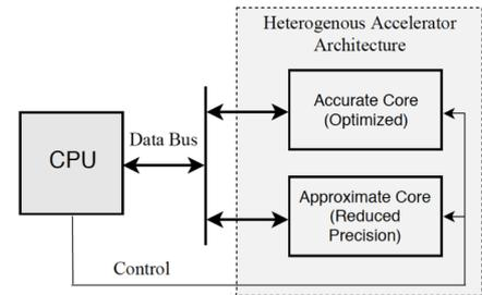
Figure 2. Our design methodology for iterative algorithms enables initial iterations to be processed on an approximate core (while the rest on an accurate core) to achieve an overall energy-efficiency.
