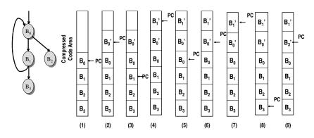
Figure 5. An example CFG fragment and the contents of the instruction memory when the basic block access pattern is  $B_0$ ,  $B_1$ ,  $B_0$ ,  $B_1$ , and  $B_3$
