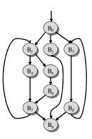
Figure 2. An example CFG fragment that can be optimized using pre-decompression
