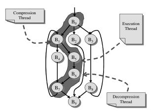
Figure 4. The cooperation between the three threads during execution. The execution thread follows the decompression thread, and the compression thread follows the execution thread
