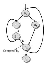
Figure 1. An example CFG fragment. Assuming that the execution takes the left branch following  $B_0$ , the 2-edge algorithm (i.e., the k-edge algorithm with k=2) starts compressing  $B_1$  just before the execution enters basic block  $B_4$
