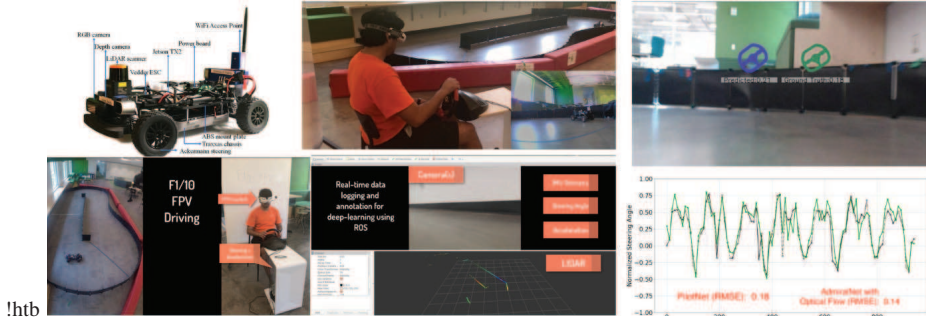
Fig. 3. The F1/10 autonomous race car setup. We can generate annotated HD images with steering and acceleration from the front camera automatically using manual driving and a first person view headset. We use ROS to automatically synchronize and label the training images.
