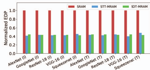
Fig. 5: Iso-area energy-delay product for NVM-based caches (lower is better) normalized with respect to SRAM-based caches for inference (I) and training (T) stages. DRAM energy and latency are also included in the results.
