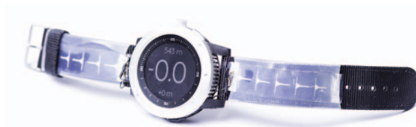
Fig. 4. Prototype of InfiniWolf where the solar panels are visible. The TEG transducer is on the bottom to touch the human wrist where it is warmer. Desing based on [21]
