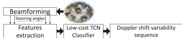
Fig. 1. System overview of ultrasonic patterns detection at the top of a microphone array.
