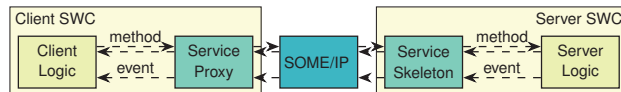
Figure 2. Communication mechanism in AUTOSAR AP. Client and server use auto-generated proxies and skeletons to communicate with their peers.
