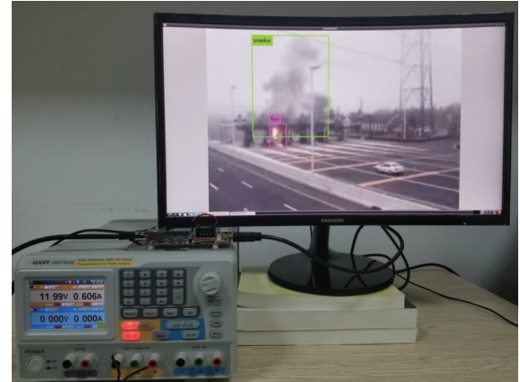
Fig. 9. Realization of the proposed framework on an ARM-core based IOT terminal device.
