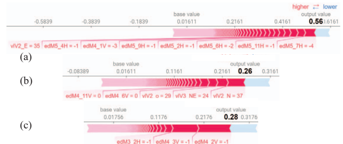
Fig. 4. (a)–(c) Most contributing features for predicting DRC hotspots in Fig. 3(a)–(c), evaluated by the SHAP tree explainer. (The blue regions on the right contain many features that are not visible as the pink bars dominate.) explanations which can be beneficial at an early design stage.
