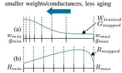
Fig. 6. Skewed weight mapping and quantization. (a) Weights are pushed towards small values, resulting a skewed distribution in contrast to Fig. 3b. (b) Resistance distribution corresponding to the skewed weight distribution.
