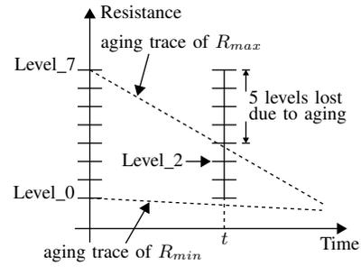
Fig. 4. Aging scenario of a memristor with the upper and lower bounds of the resistance range decreasing with programming time.
