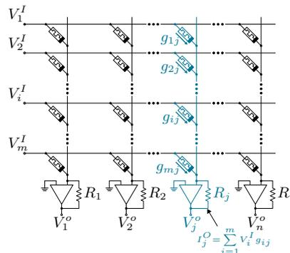
Fig. 1. Memristor crossbar architecture.
