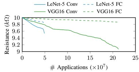
Fig. 11. Aging of convolutional layers and fully-connected layers.
