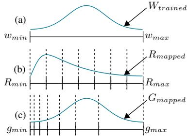
Fig. 3. Hardware mapping and quantization. (a) Weights after software training. (b) Resistance distribution after mapping with quantization. (c) Conductance distribution after mapping with quantization.
