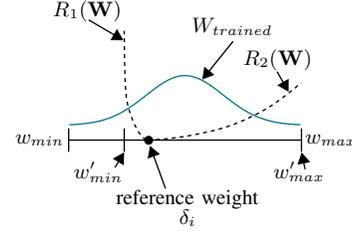
Fig. 7. Regularizations in skewed weight training.  $\mathbf{W}^{trained}$  is the distribution of the original weights.  $R_1(\mathbf{W})$  and  $R_2(\mathbf{W})$  are the new terms for the cost function to generate skewed weights. With these regularizations, a skewed weight distribution as in Fig. 6(a) can be generated.
