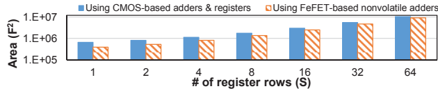
Fig. 10: Area comparison between the cases using CMOS- and FeFET-based adders and registers respectively.
