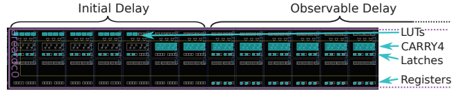
Fig. 3: Floorplan (rotated right) of one TDC Sensor with 18 \times (\text{LUT, Latch}) as part of the Initial Delay.
