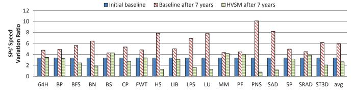
Fig. 5. SPs' speed variation ratio comparison: the initial baseline, baseline after seven years of execution and HVSM after seven years of execution.
