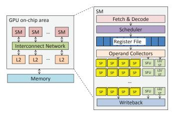
Fig. 1. GPU architecture (SM: streaming multiprocessor; SP: streaming processor; SFU: special function unit; LD/ST: load store unit).
