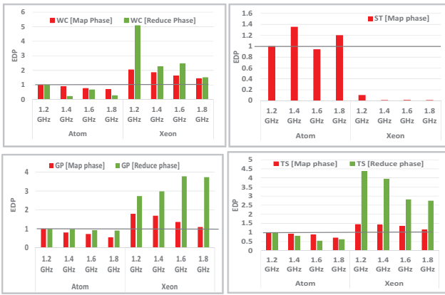
Figure 5: EDP analysis of Map and Reduce phase of (a) WordCount (b) Sort (c) Grep (d) Terasort on big and little core with frequency scaling
