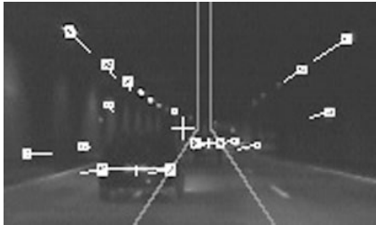
Fig. 2. Final output image of the system. Markers show all detected lights, their motion vectors and detected vehicles.
