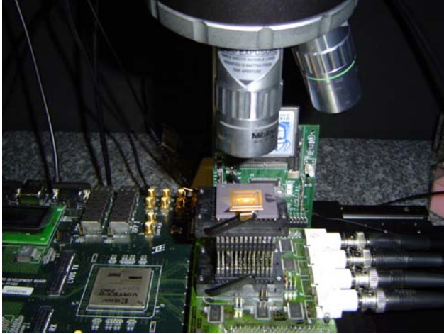
Figure 5: Laser platform with the Montgomery demonstrator test board.
